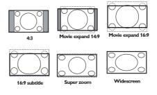
Super Zoom, Movie expand 14:9, Movie expand 16:9 and 16:9 subtitle makes the picture fill the screen as much as possible. It is recommended to press the cursor up/down key to adjust the picture position on the screen.
